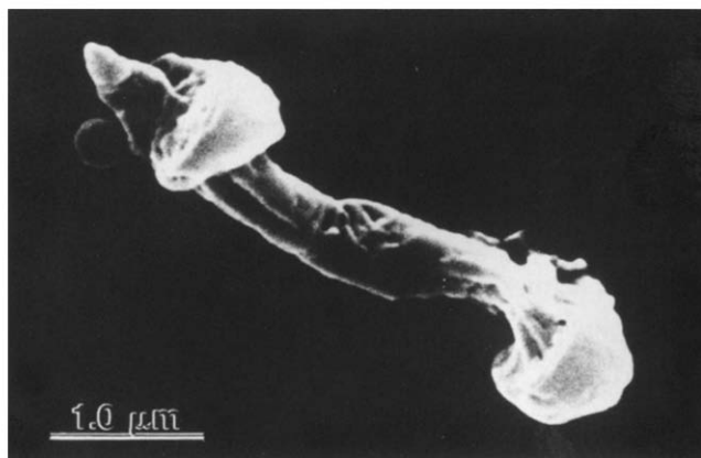
Figure 2 Scanning electron micrograph showing a highly deformed granule. The smeared core remains attached to the shell fragments of the granule. The deformation conditions are the same as for Figure 1
